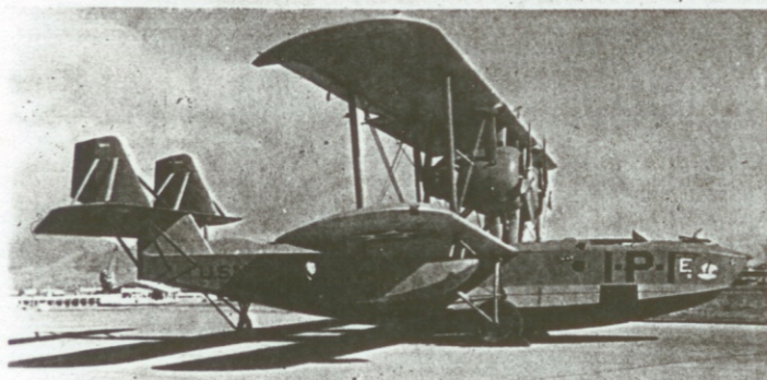
A PLANE OF SQUADRON VP-1F MODEL PM-1 BOAT TYPE SEAPLANE HAS GASOLINE CAPACITY FOR ABOUT TWELVE HOURS DISTINGUISHING CHARACTERISTICS TWIN VERTICAL RUDDERS HULL PAINTED DARK GREY TAIL SURFACES PAINTED RED
